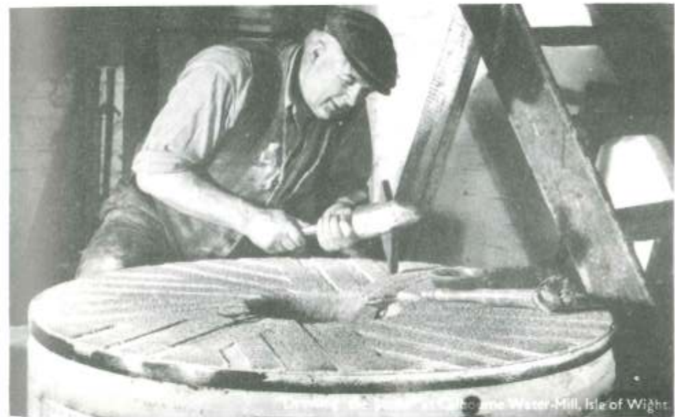
Mr. J. Weeks dressing a millstone with a mill bill at Calbourne Mill, Isle of Wight. The wedge-shaped tool for cutting the grooves is set in a thrift. This tool would have been used by Richard Huxtable.
